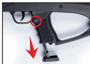
Push the magazine release button and pull out the magazine.
