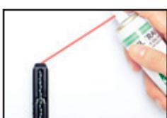
Add a few drops of silicone oil on the BB located in the BB loading hole. Reinsert the magazine into the Airgun.
